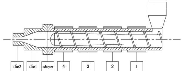
Type: screw: 45mm, L/D: 30, compression ratio 3:1
